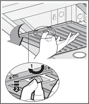
**Fig.2:** Remove the buffle filters by pulling the lever **1** out and pushing downwards **2**.
