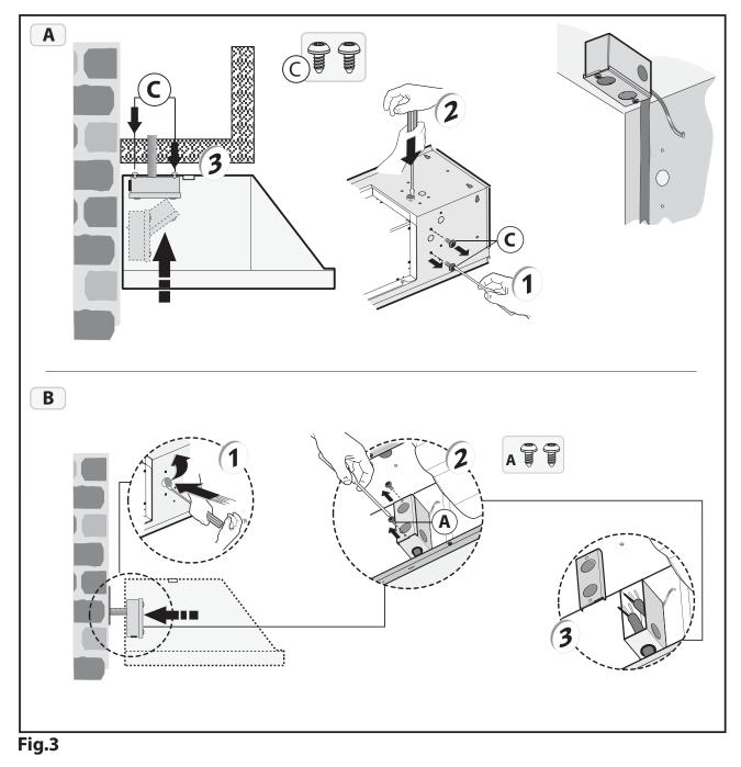
• The appliance must be installed at a minimum height of 27" from an electric cooker stove, or 32" from gas or combined cooker stoves. If a connection ductwork composed of two parts is used, the upper part must be placed outside the lower part. Do not connect the range hood exhaust duct air to the same duct air used to exhaust hot air or fumes from other appliances other than electrical.
