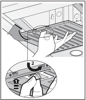
**Fig.5:** Put the buffle filters back in place (**Fig.2**).
