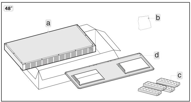
**CARBON FILTER KIT XORFK09 (48"):** We have an air diverter **A**, 7 screws **B**, 4 rectangular filters **C** and the bracket **D**.
