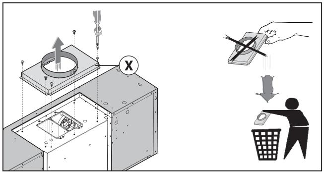
**Fig.1:** Take the circular shape **X** and fasten it to the hood using the 7 screws. To convert this model from the sunction to the filtering version, it is not necessary to use the circular shape **X**.
