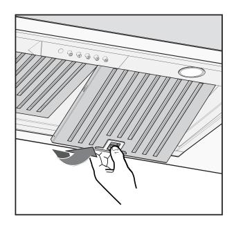
frequently. Use a warm detergent solution. Grease filters are a dishwasher safe.
