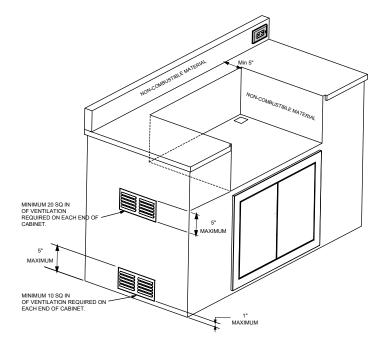
Natural Gas is lighter than air. Vents should be placed 10" below the countertop.
