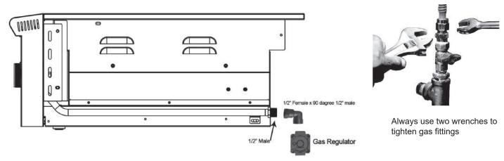
Use plumbers putty or gas tape on the male threads to seal the male threads to seal the connection.
