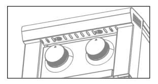
2 Remove the LED light assembly and disconnect it from the power connector.
