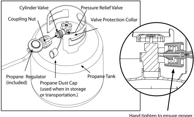
Hand tighten to ensure proper seal for correct gas flow.
