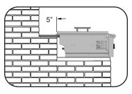
No materials shall be used within 12" of the unit that will burn or be affected by the high heat the unit can produce.
