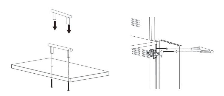
Remove the right side shelf from the cart and place in a safe place for installation to side burner cart. Remove the right side shelf brackets for installation on the Side Burner Cart.
