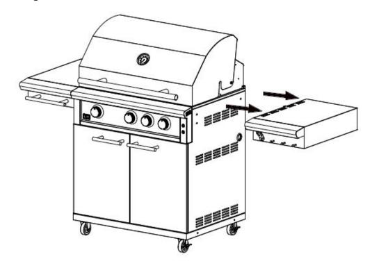
Screw into the right side panel and base 6 - M5x10 bolts 2/3 of the way in as shown below.
