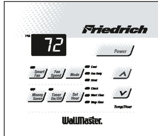
Figure 6: "WE"/"WY" heat/cool models Electronic Control Panel
