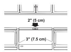
Allow at least 3 in. (7.5 cm) of air space on both sides of the freezer and 2 in. (5 cm) between the back of the freezer and the wall. Leave room above the freezer to open the lid.
