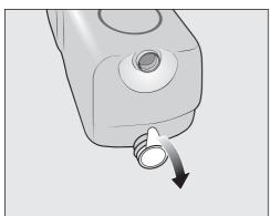
Remove the film seal from the cartridge completely.
