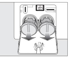
Remove the drain filters completely.
