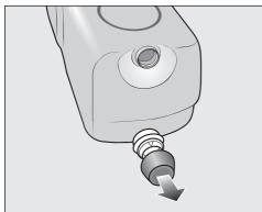
Remove the cover cap from the cartridge.
