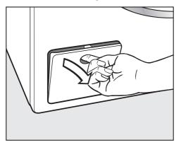
Open the drain pump flap.
