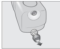
Remove the cover cap from the cartridge.
