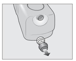
Remove the cover cap from the UltraPhase 1 detergent cartridge included with the delivery.
