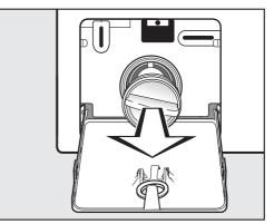
Remove the drain filter completely.
