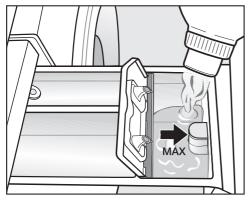
Add the fabric softener or the liquid starch to the & compartment. Do not exceed the maximum level mark.
