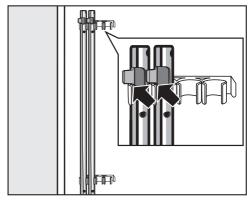
Secure the shipping struts to the back of the washing machine. Make sure that the top catch is located above the holder.
