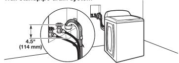
See requirements for floor standpipe drain system.
