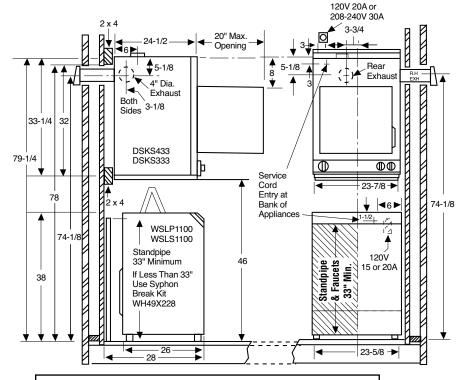
(†) Exhaust 4" Dia. Exhaust Both Sides 3-1/8 32 33-1/4 DSKS433 DSKS333 73-1/4 <u>ФФ</u> Service Cord Entry at Bank of 68-1/8 Appliances -WSLP1100 68-1/8 Standpipe 120Ý 33" Minimum 15 or 20A If Less Than 33" Use Syphon Break Kit WH49X228
