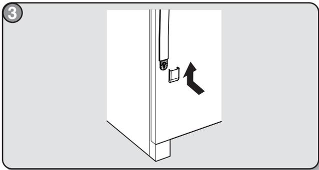
Tighten all screws completely plus an additional quarter-turn. Install the screw cover.
