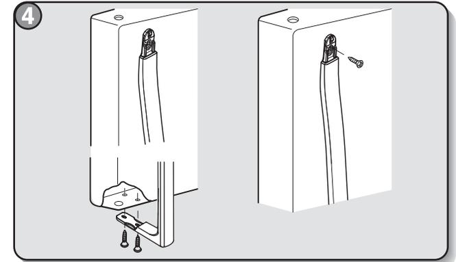
Align the second handle with door screws and push the base firmly against the door. Partially tighten the screws (2 turns).
