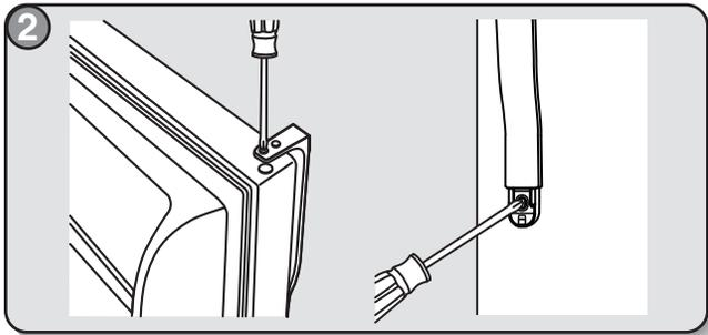
Align one of the handles with door screws and push the base firmly against the door. Partially tighten the screws (2 turns).
