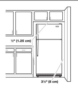
To ensure proper ventilation for your refrigerator, allow for a  $\frac{1}{2}$ " (1.25 cm) space on each side and at the top. Allow at least 2" (5.08 cm) between back of cabinet and the wall. If your refrigerator has an ice maker, make sure you leave some extra space at the back for the water line connections.
