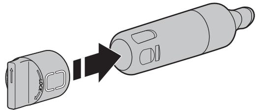
6. Insert the filter into the housing.
