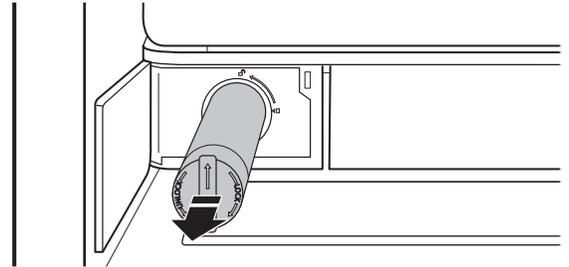
4. Remove the water filter cap from the water filter.
