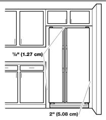
To ensure proper ventilation for your refrigerator, allow for ½" (1.27 cm) of space on each side and at the top. Allow for 1" (2.54 cm) of space behind the refrigerator. If your refrigerator has an ice maker, allow extra space at the back for the water line connections. When installing your refrigerator next to a fixed wall, leave a 2" (5.08 cm) minimum space on each side (depending on your model) to allow the doors to swing open.
