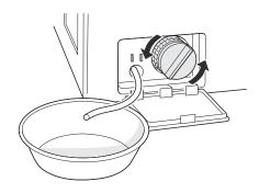
**5** Clean the pump filter and opening.
