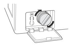
Close the drain pump filter cover.
