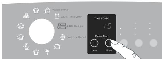
Fig.28 Modifying the number of beeps to signal the end of the cycle
