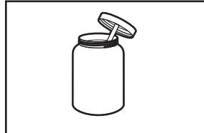
Pipe-joint compound resistant to LP gas
