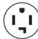
4-wire receptacle (14-30R)
