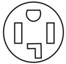
4-wire receptacle (14-30R)
