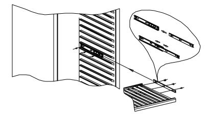
? To remove the shelves out of the rail pull each shelf approximately 1/3 out. Use a long flat screwdriver to press down the right plastic notch as shown in Figure A and at the same time lift the left plastic notch as shown in Figure B. Then proceed to pull out the shelf slowly. Contact our service department if assistance is needed.
