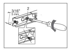
Partly (by no more than 5 mm) undo the hinge screws (2) at the top and bottom. Do not completely undo the screws. This way, the door will remain in contact with the housing.
