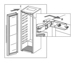
10. Hang the door onto the screws (2) at the top and bottom and slide it in the direction indicated by the arrow (a).
