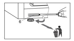
7. Remove the cap (6) and discard into the bin for plastic waste.
