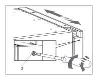
Close the door, then rotate the screw (2) at the top and bottom to adjust the door position.
