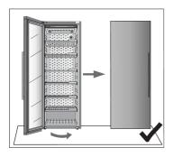
Adjust the door position until the edge of the door is parallel to the side of the housing.
