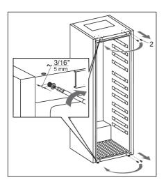
8. Completely undo the screws (2). Then, partly screw them into the holes at the top and bottom on the opposite side of the housing.
