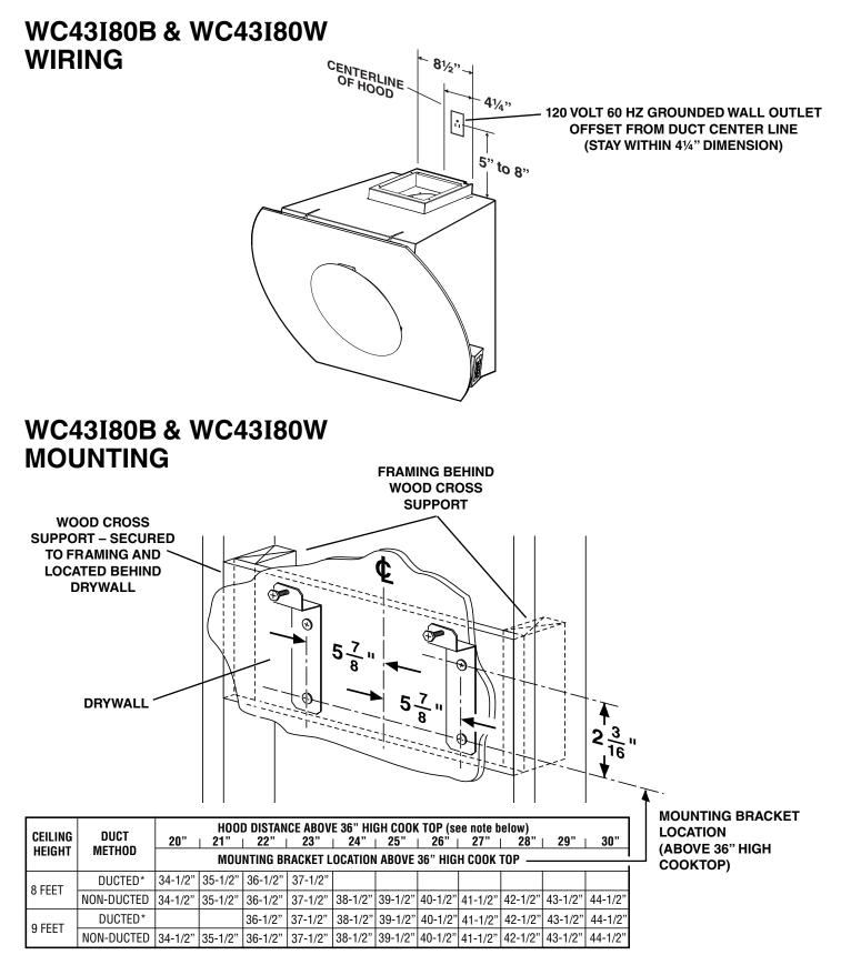
Note : Minimum hood distance above cook top must not be less than 20". A maximum of 30" above cook top is highly recommended for best capture of cooking impurities. Distances over 30" are at the installer and user's discretion; and if ceiling height and flue length permit. \* Ducted hood requires the purchase of flue kit model AEWC43SP.
