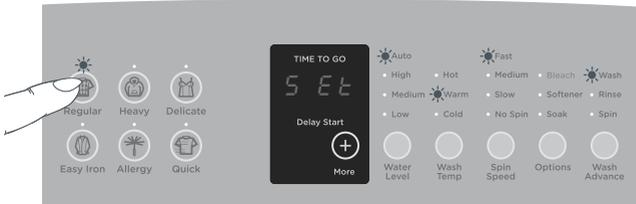
Fig.31 Customizing a wash cycle, eg REGULAR cycle
