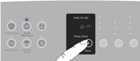
Fig.36 Changing the out of balance recovery routine
