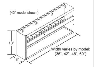
This Fire Magic Spacer is specifically designed for your Fire Magic Vent Hood. To install, read and follow <u>all</u> instructions in the owner's manual provided with your vent hood.
