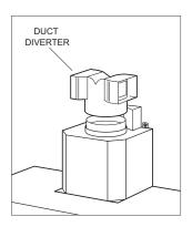
Install the diverter extensions on both sides of the duct diverter.
