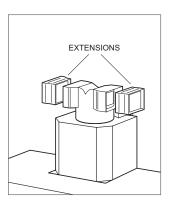
3 Place the lower chimney on the hood so the diverter extensions align with the vent holes in the chimney.
