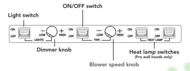
**Fan On/Off switch**—Starts and stops the blower. When turned on the blower will operate at the previous setting of the speed control.
