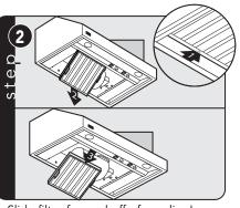
Slide filter forward off of rear lip. Lower filter rear, then slide filter front out.
