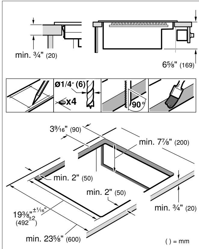
**Flush mounting:** Flush mounting into a countertop is possible.
