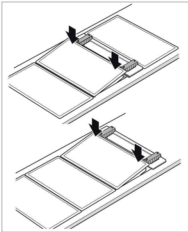
**4** Fit the connection piece in the required position.
