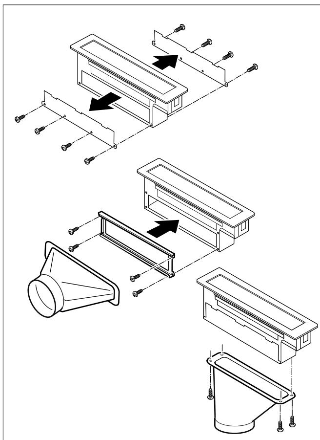
**5** Secure the exhaust air pipe to the connecting pieces and seal appropriately..
