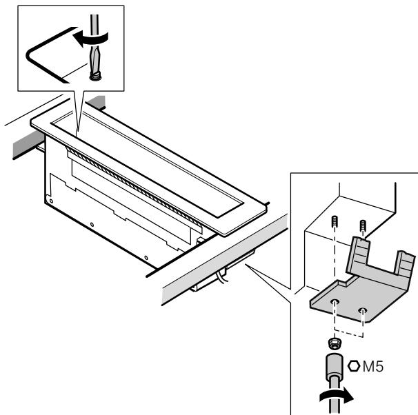
**3** Use the installation aid. Horizontally insert the downdraft ventilation unit in the recess and align it. Remove the sealing element. Insert the installation aid at an angle into the ventilation recess and align it vertically to the appliance. Position the appliance at an angle in front of the downdraft ventilation unit and press it into the recess via the installation aid. Remove the installation aid. Fasten the downdraft ventilation unit as described above.
