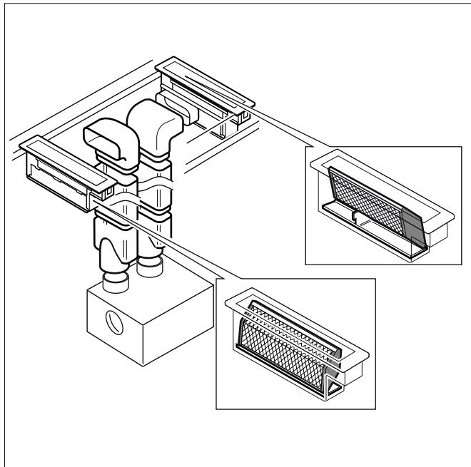
For downwards air outlet, place the grease filter without the positioning plate in the ventilation element. The alignment of the grease filter does not matter.
