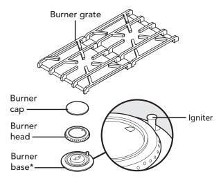
\*Note: When replacing burner head, carefully align the tab underneath the cap with the slot in the burner base.
