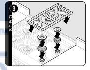
Burner heads and burner bases are packed in cardboard top pack with the grates. Place the burner base on top of the burner flange and the burner head on top of the burner base. Place burner grate on top of grate support.
