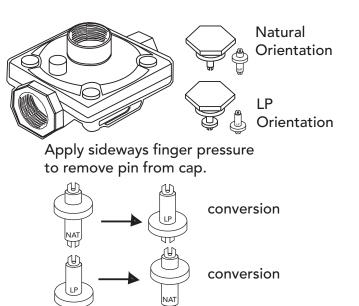
**NOTE:** VGR748 models have two regulators. Make sure both regulators are converted. To access second regulator, the island trim and small panel on the back must be removed
