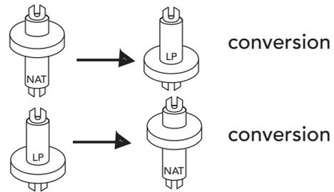
**NOTE:** VGR748 models have two regulators. Make sure both regulators are converted. To access second regulator, the island trim and small panel on the back must be removed
