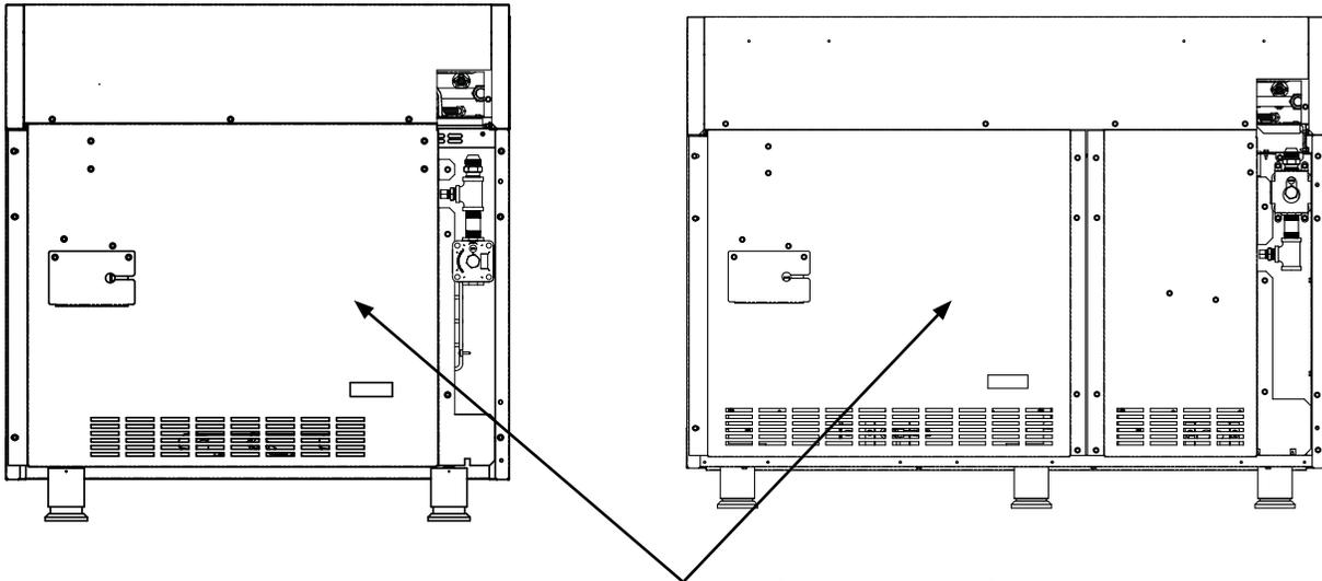
Remove rear panel to access infrared broiler orifice.
