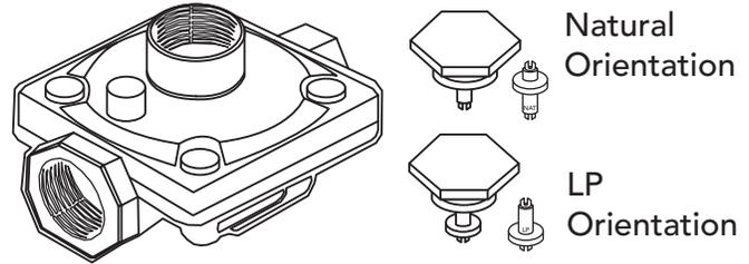
Apply sideways finger pressure to remove pin from cap.
