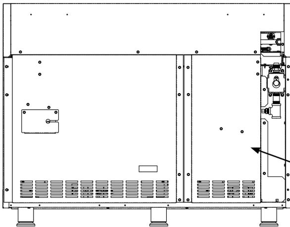
Second regulator located behind small panel on VGR748 Gas Ranges.
