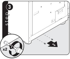
Remove two screws from back of range.
