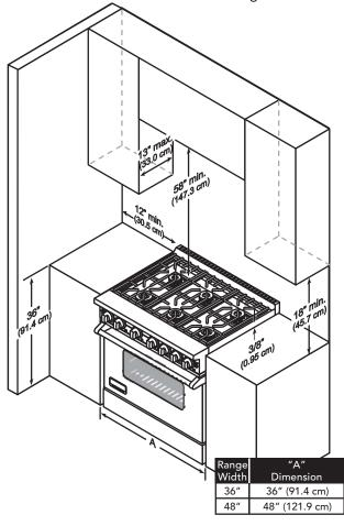
**Note:** Minimum clearance for back wall is 3/4" (1.9 cm) with backguard or high-shelf.
