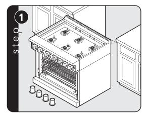
Legs are packed in cardboard top pack. **Note:** Legs should be installed near to where appliance is to be used, as they are not secure for long transit.
