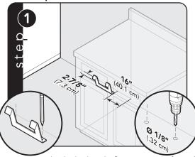
Locate anti-tip bracket hook on the floor 16" 40.1 cm) from side cabinet and 2-7/8" (7.3 cm) from rear wall. Mark and drill 1/8" (.32 cm) holes where bracket will be located.
