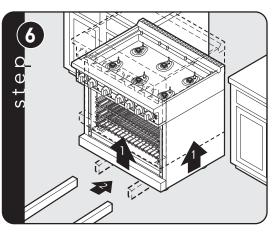
Lift unit and prop on wood blocks.
