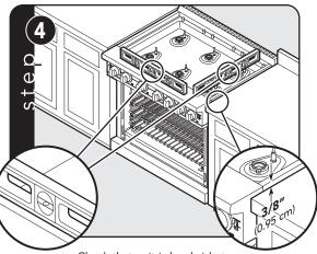
Check that unit is level side to side and front to back. Side trim of the lowest corner must be 3/8" (0.95 cm) above countertop.
