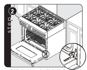
Fold latches backward until locked in place
