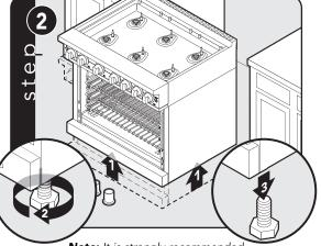
Note: It is strongly recommended that a pallet or lift jack be used rather than tilting. Raise unit about a foot. Unscrew shipping bolts from couplings on all four corners.
