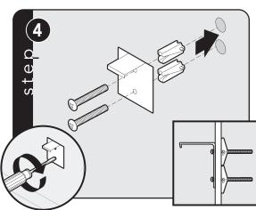
Attach bracket with mounting hardware provided.
