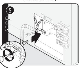
Attach ground lead (green) with ground screw that was removed.
