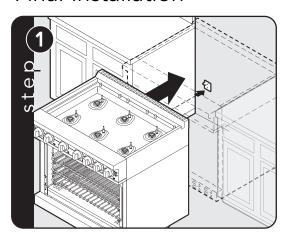
Slide range into place. Be sure wall anit-tip bracket slides into the anit-tip opening and floor anti-tip hook and bracket are engaged.
