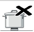
Place the pots on the pan supports, never directly onto the burners.
