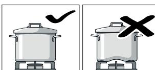
Don't use any deformed cooking vessels that don't stand solidly on the stovetop. The vessels could tip over.
