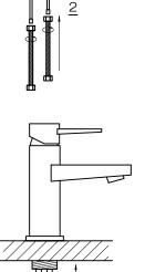
4. CONNECT FLEXIBLE HOSES TO THE COLD AND HOT WATER SUPPLY.
