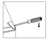
2.Undo the screws.Then remove the hinge bracket.
