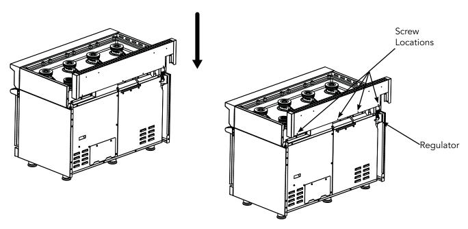
**NOTE:** Regulator will be visible after rear trim accessory is installed.
