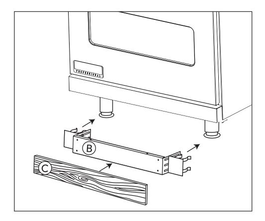
**Important Note**: The range must be installed as specified in the range installation guide for proper airflow when using the custom curb base.
