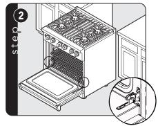
Fold latches backward until locked in place.
