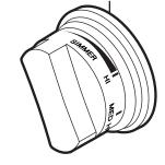
Within a few moments, enough gas will have traveled to the burner to light. When the burner lights, turn the burner control to any position to adjust the flame size. Setting the proper flame height for the desired cooking process and selecting the correct cooking vessel will result in superior cooking performance, while also saving time and energy.
