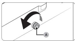
1. Open the door that is closer to the main body than the others. Then, turn the adjustment dial (A) counterclockwise until the gap becomes even with the others.
