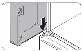
1. While holding the door open by more than 90 degrees, insert the shaft on the middle hinge into the hole on the bottom of the door.
