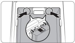
2. With the left Showcase door open, open the fridge door. Then, push the upper part of the Beverage Zone (left and right side of the fan) from inside to release the snap joints securing the Beverage Zone cover to the door.
