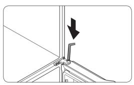
**4.** Locate the hinge shaft. While holding the door with one hand, use a flat-head screwdriver or Allen wrench to press the shaft down. Make sure to hold the door to prevent the door from falling.
