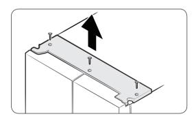
**1.** With the doors closed, use a Phillips screwdriver to remove the screws (x3) from the top cover. Pull up and remove the top cover with the connectors.
