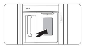
To dispense chilled water, open the Beverage Center and press the dispenser lever.
