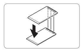
**4.** If you need to further raise the rear height, attach another adjustment pad on top of the first level adjustment pad.
