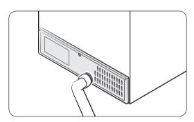
To keep cords and exposed parts of the rear panel free of dirt, vacuum the panel once or twice a year.
