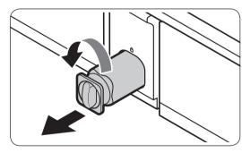
3. Turn the knob of the filter cartridge counter clockwise 90 degrees (1/4 turn). The filter cartridge unlocks.
