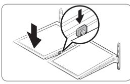
• To remove a shelf, fully open the corresponding door. Hold the front of the shelf, and then gently lift up and pull out.
