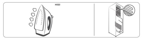
As the refrigerator cools or freezes, refrigerant gas moves through sealed pipes, causing bubbling sounds.
