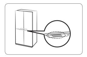
Touch the sensor near the door handle of the fridge. The door will open.
