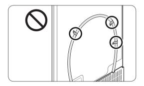
Do not mount the water filter or water line on any part of the refrigerator. This may damage the refrigerator.
