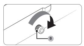
2. After adjusting the gap, turn the locking nut (B) to lock the adjustment dial.
