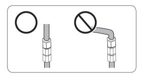
• If you have to relocate the refrigerator after connecting the water line, make sure the joined section of the water line is straight.
