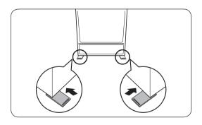
If you need to raise the rear side of the refrigerator to level it, you can use the provided level adjustment pad(s). Follow these instructions to raise the rear side of the refrigerator.
