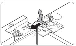
**2.** Disconnect the two wire connectors on the left door. The position of the connectors differs with the model.
