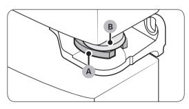
2. Insert a suitable-sized snap ring (A) between the door grommet (B) and the hinge as shown.
