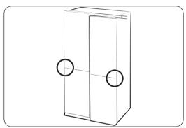
1. Check the height difference between the doors, and then lift up and hold the door with the lower height.
