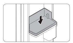
1. With the fridge door or the Showcase door open, align the grooves on the left and right side of the bottom door bin, and then insert it.
