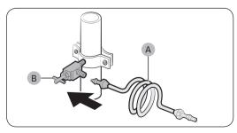
3. Connect the water line installation kit (A) to the shutoff valve (B).
