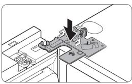
**2.** Put the top hinge into position on the top of the refrigerator, and then insert the hinge shaft into the top hole of the door. Make sure the wires from the door pass through the hole in the hinge shaft.
