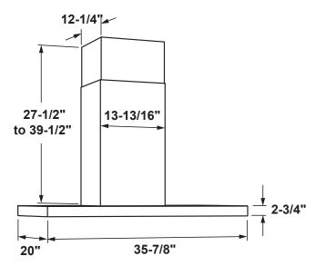
36" models require a 36"-wide opening \*The supplied duct cover fits 7'-7" to 9'-6" ceiling heights (10' ceiling height with optional high ceiling kit UX10DC83SS) (12' ceiling height with optional high ceiling kit UX12DC93SS) (14' ceiling height with optional high ceiling kit UX14DC93SS)
