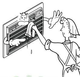
**When the unit is to be cleaned, switch off, and turn off the breaker.**
