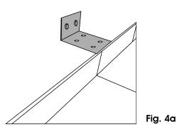
OPTION 1: wall mounted bracket ATTENTION: check that the cooker is leaning against the rear wall to avoid tipping.
