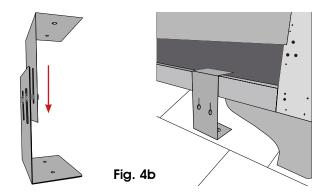
OPTION 2: floor mounted bracket ATTENTION: in this case 2 brackets are needed
