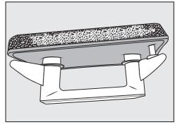
Residues arise from laundry fibers and traces of detergent components. They can be found on the front and side edges of the plinth filter. In extreme cases, they can form stubborn crust. Residues are a sign that the plinth filter no is longer a snug fit at the sides, even if it appears to be perfect:
