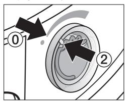
■ Turn the outer ring counterclockwise until marker ② is in position ⑨.
