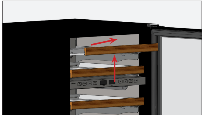
FIG. 1. Lift and pull the wine rack forward.
