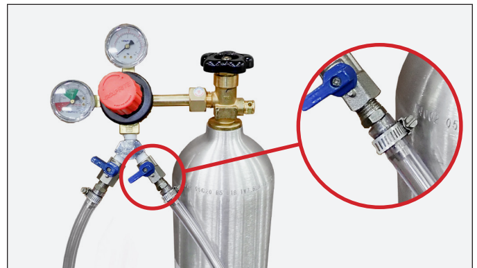
FIG. 7. Installed pressure regulator and air hoses. Be sure the hose clamps are tightened to prevent leaks.
