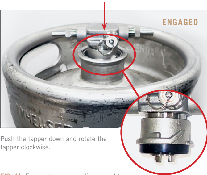
FIG. 11. Engaged taper vs. disengaged taper
