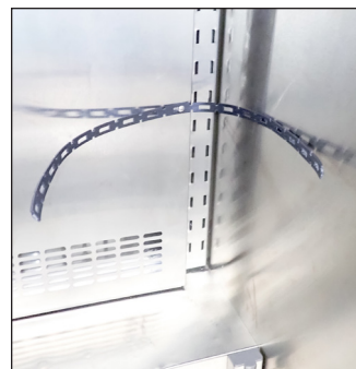
FIG. 8. Installed safety strap.
