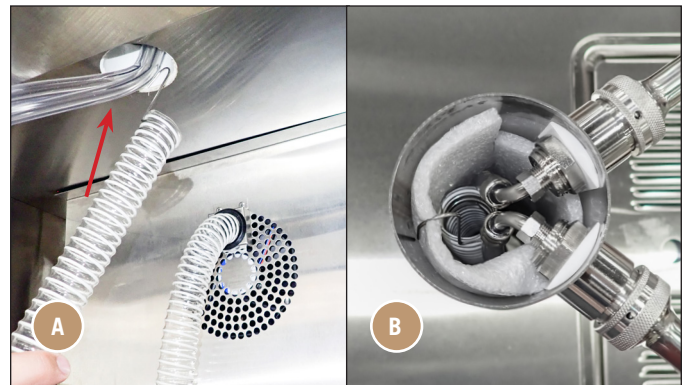
FIG. 6. Route the chill hose into the draft standard from below (A) and hook it on the top of the insulation sleeve (B).
