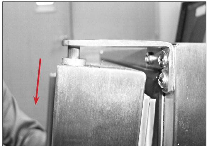
FIG. 3. Lower the door off the top hinge.
