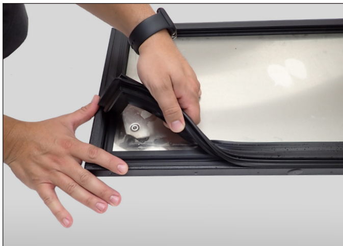
FIG. 3. Pull the gasket from the drawer.
