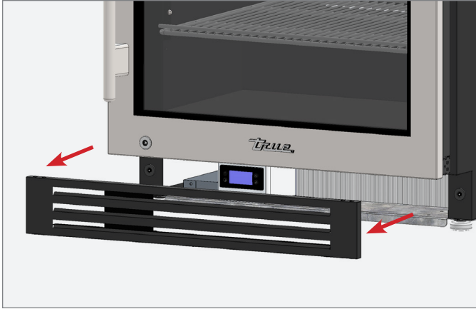
FIG. 1. Pull the kickplate off the magnets.
