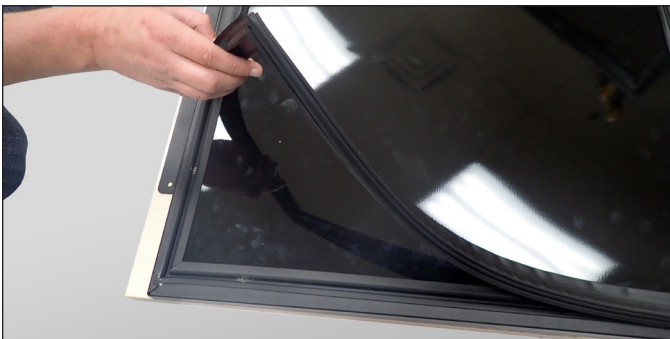
FIG. 3. Pull the gasket from the door.
