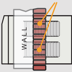
ROOM AIR CONDITIONER BLOCKED SIDE VENTS RESTRICT AIR FLOW
