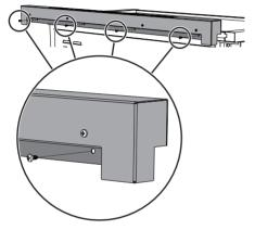
2. Secure the backguard to the top by tightening screws.
