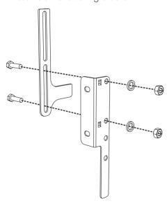
3. Align the base of the hook on the fastening bracket with the base of the slot on the wall fastening plate.
