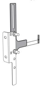
4. Align the base of the fastening bracket with the ground and tighten the screws to fix the measurements.
