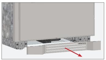
FIG. 1. Pull the kickplate from the cabinet.
