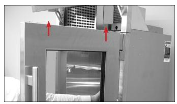
FIG. 3. Lift the door up.
