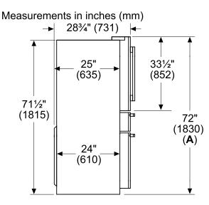
A: Add <sup>5</sup>/8" (17) with front leveling feet fully extended
