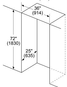
Leave  $\frac{1}{2}$ " (12.7) gap at the top and 1" (25.4) behind the refrigerator for proper ventilation.
